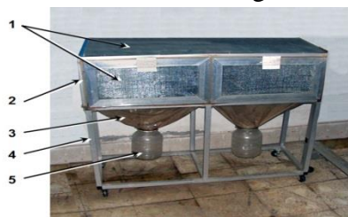
Figure (1): Two of the cages used for the mass rearing of Sitotroga cerealella . 1. Steel mesh, 2. Upper part of the cage, 3. Funnel, 4. Metal stand and 5. Collecting plastic jar.
