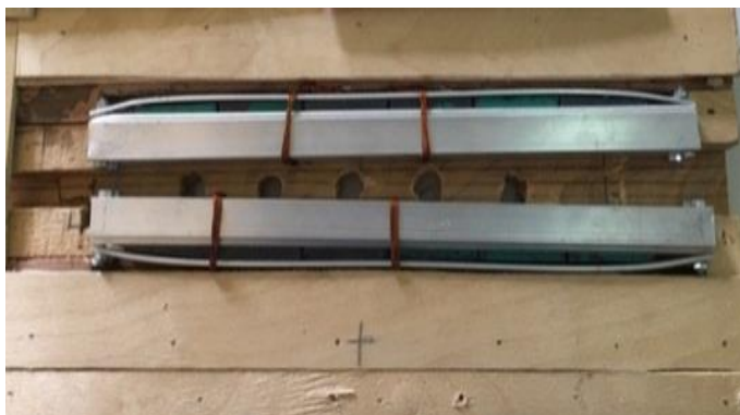
Figure (1): Apparatus consists of 2 rows inside each row 8 magnetic pieces.
